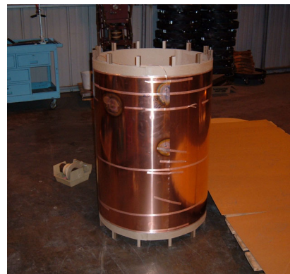
Figure 26. Example of power factor model used in tests to evaluate dry air transport of Envirotemp FR3
