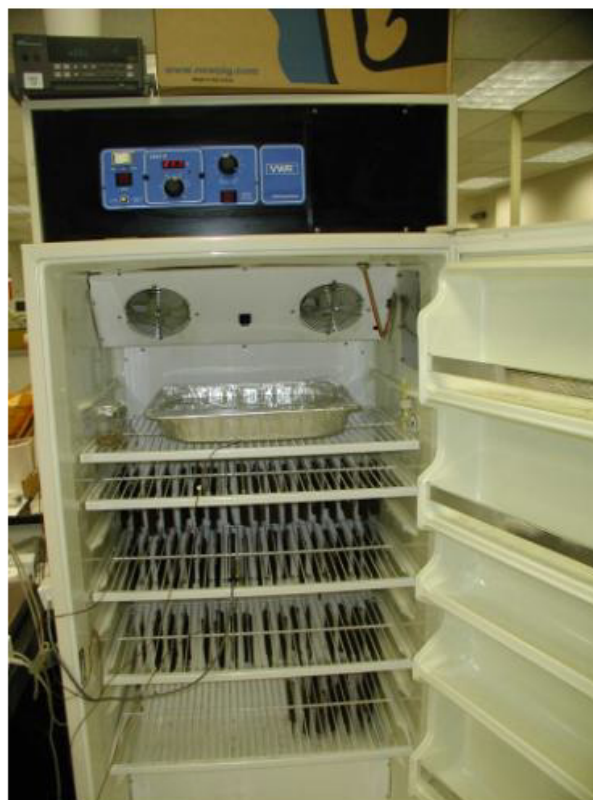
Figure 1 Chamber used to equilibrate the water content of the previously aged Kraft paper. Fans inside the chamber circulate the air to stabilize the humidity throughout and assure consistent exposure of all specimens. Sensors continuously monitor temperature and humidity.
