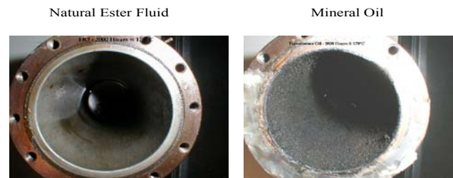
Fig. 4. Interior of aging tubes after 2000 hours at 170°C [10].
