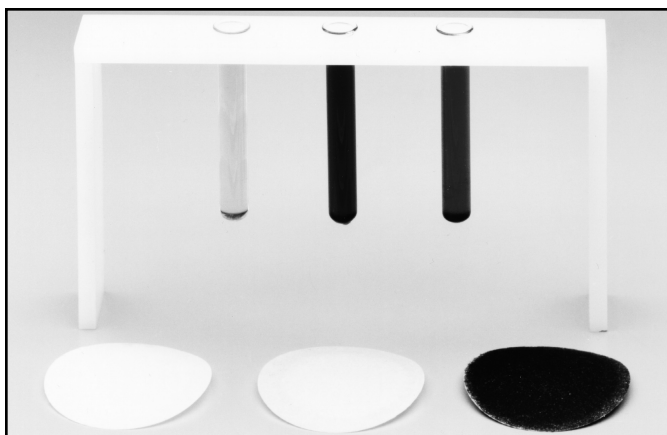
Left to right: Envirotemp FR3 fluid, R-Temp® fluid and Conventional Transformer Oil after 120 hours at 165°C.
