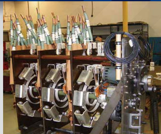
GE LRT-72 Load Tap Changer Training Model
