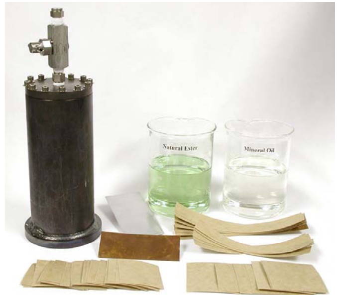
Fig. 1. Components of a sealed test system.
