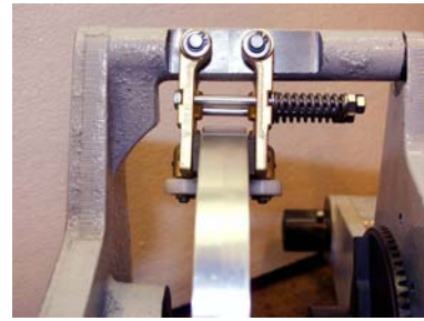
Figure 3: Dual Nylon Rollers open the brakes by riding up and out of the cam slots on the flywheel. During scheduled service intervals, inspect and clean flywheel and nylon rolling surfaces
