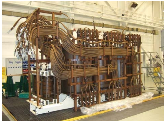
FIG. 2 - Transformer designed with a preventive auto transformer for use with 2,500A reactance bridging load tap changer.
