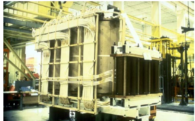
FIG. 1 - Transformer designed with a series transformer (at right end) for use with 600A resistance bridging load tap changer.
