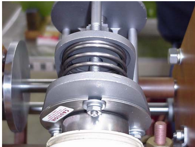
Fig. 2: Alignment of stud through upper actuator arm
