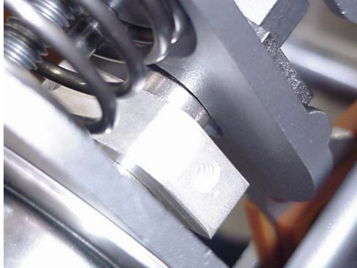
Fig. 3: Alignment of vacuum interrupter shaft through upper actuator arm
