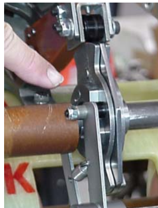
Fig.5: Dual-slope and Auxiliary Control Cam Assembly
