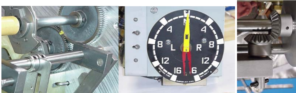
Fig. 3: Paint marks on drive gears match up, position indicator on neutral, and bevel gears meshed with set screw tightened,
