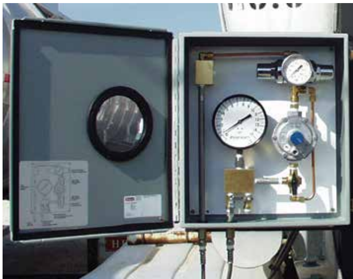
Supply and tank pressure gauges on the Mini Inert Air System are easily viewed through a large viewing port on the cabinet door.
