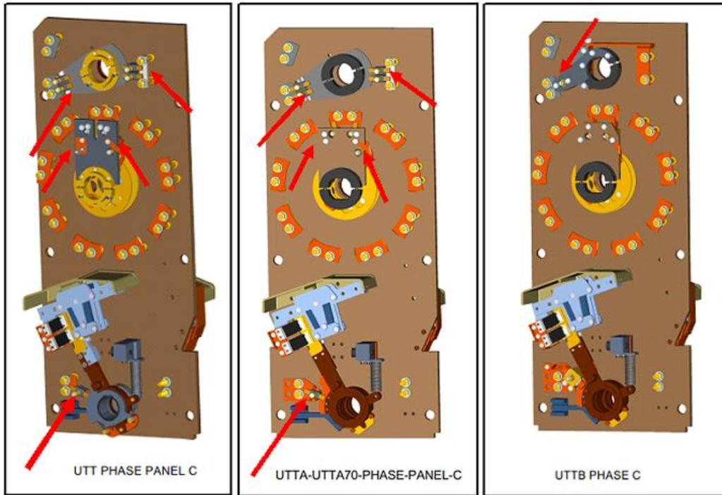
Below is a different view of the moving selector switches for the UTT-A/A70 and UTT. Red arrows again point out common areas most affected by overheating and coking.
