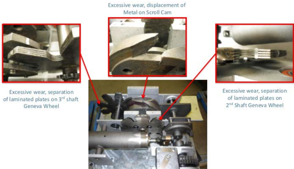
Figure 5: Wear Patterns on Geneva Wheels and Scroll Cam
