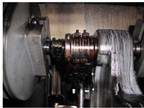
Film on Reversing Switch Contact
