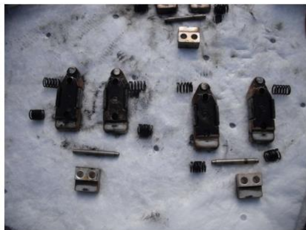
Early stages of coking on Reversing Sw Springs
